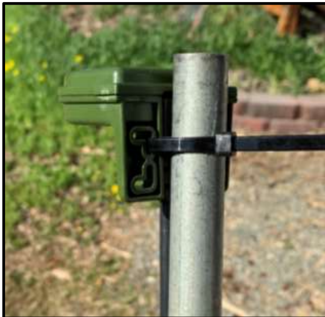
Figure 2. SM-U2 microphone used for SM4 units secured to the conduit with a zip tie
