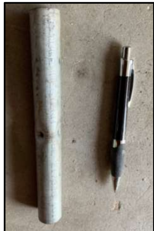
Figure 1 Home-made coupler made from 3/4 inch conduit crimped in the middle used to connect the two pieces of the mast. Pen for scale.
