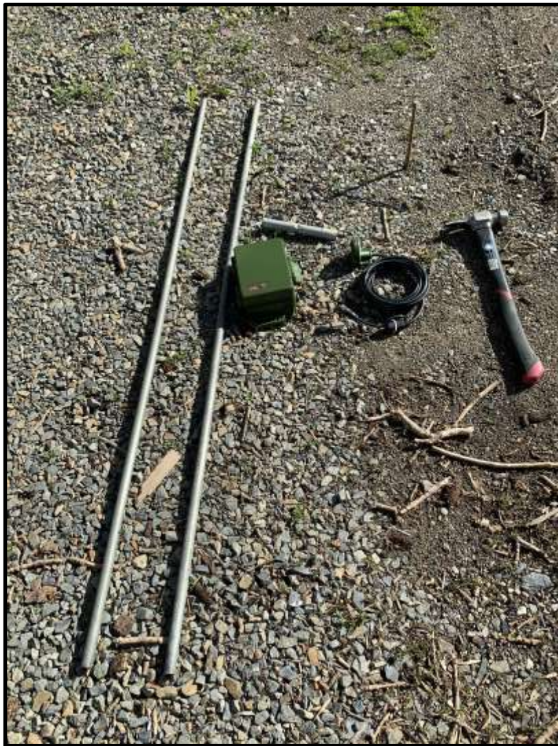
Survey Equipment. Two pieces of conduit, a connector, rebar, hammer, detector, and microphone
